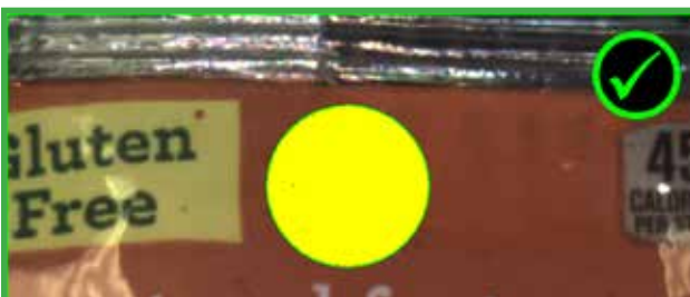
Color pixel count tool confirms the integrity of packaging by identifying pixel values of colors trained in the region of interest.
